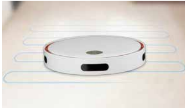
Cleaning path in automatic cleaning mode
